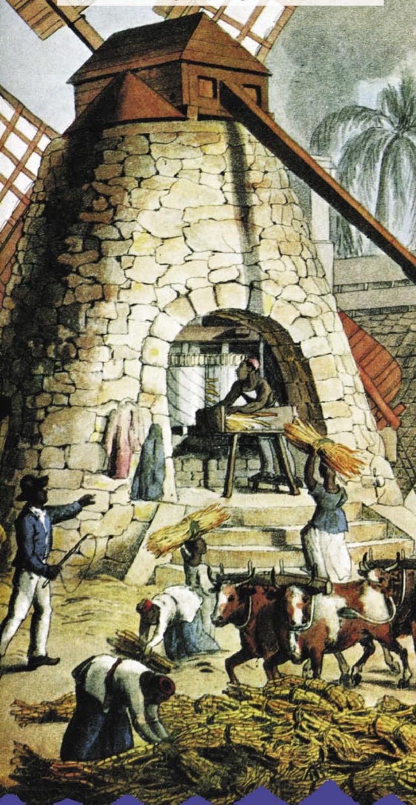
3 Carts transport the cane from field to windmill – the crusher squeezes the juice out of the cane, the mangled stalks are used to stoke fires at the boiling-house and distillery
