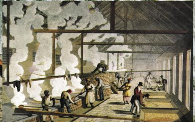
4 Slaves ladle steaming juice from vat to vat and clear it of the scum, a gutter leads the boiling liquid into cooling trays
