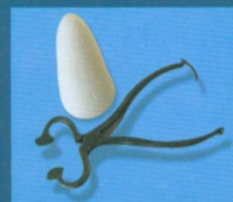
Sugar nippers became commonplace to cut the sugar cones which came from the West Indies.
