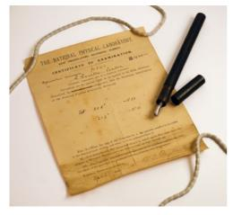
Hypsometric thermometers were used to determine height above sea level by measuring the boiling temperature of water at different heights. The changing boiling points are a result of the difference in air pressure the higher one is above sea level. These specially crafted thermometers, with their apparatus, were used by Grenfell and other explorers to plot the height of mountains and hills.
